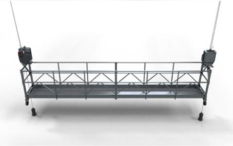
The supporting structure of the platform is welded from high-quality steel profiles, the floor is made of aluminum sheeting with anti-slip treatment. The individual sections are assemled to the target length with bolts and self-locking nuts. The platform is equipped with wheels to move the platform around the construction site.
